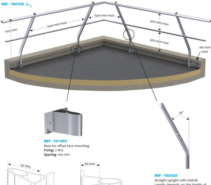
Straight upright with midrail. Length depends on the height of the parapet.
