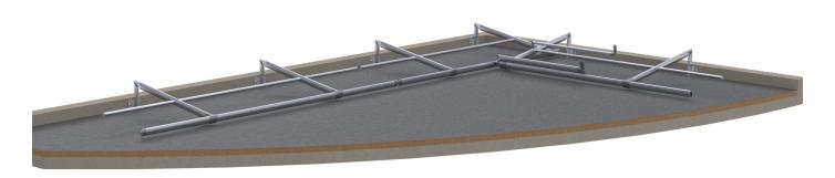
Fold down the guardrail section towards the inside of the device. Do the reverse operation to put the **SECURILISSE**® in operational position.
