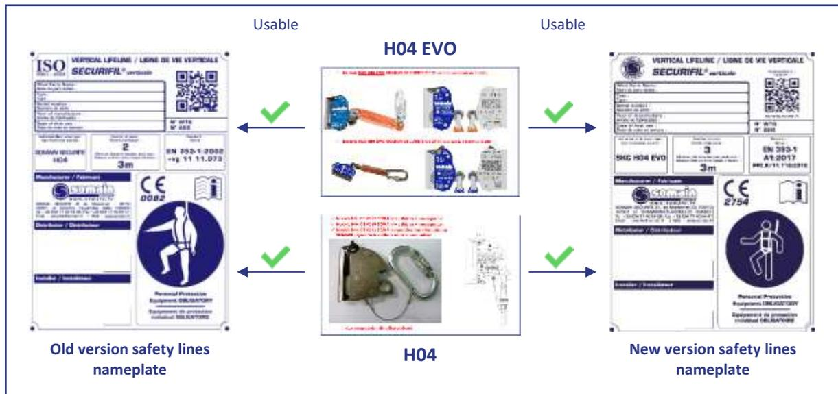
In order to specify the versions of the runner compatible with the safety lines and to avoid confusion on site: we have developed an additional nameplate to be installed below the current mandatory nameplate (as per diagram below).
