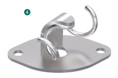
**REF : 102270** V2 inox intermediate part. Every 15 metres maximum. **Centre-to-centre distance:** 2 holes 141 mm.
