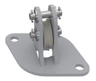
REF : 102188 v2 inox pulley. Every 15 metres maximum. 2 holes. Centre-to-centre distance: 141 mm Fixing: M10 or M12
