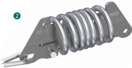
REF : 102173 Aluminium/stainless steel eye shock absorber, installed at one end of the lifeline, reduces stress on the structure in case of a fall. Traceability by unique serial number. Equipped with a tension and fall indicator.
