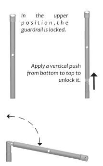
Then tilt the upright to the lower position. Do the operations backward to put the
